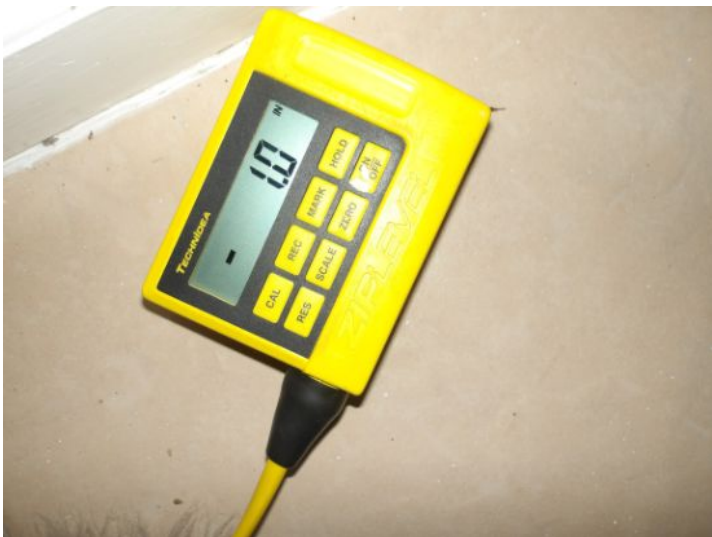
Structural movement and/or settling noted in Back Building. Suggest that a licensed professional be consulted for further evaluation.
