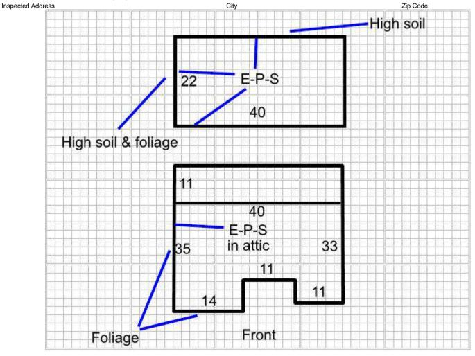
Additional Comments An ACTIVE Infestation of termites was discovered at the time of this inspection. See diagram for location(s). Treatment Recommended., There is visible evidence of a previous WDI infestation at the time of this inspection without signs of previous treatment or records of previous treatment. Treatment is recommended at this time. See diagram for location(s).
