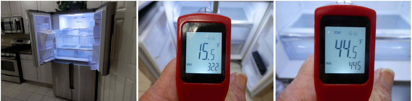
checking the temperatures at the freezing and cooling sides
