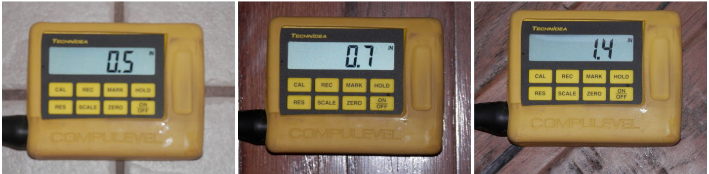
a sample of the comp-u-level measurements taken at various locations on the floor (see graph for additional measurements)
