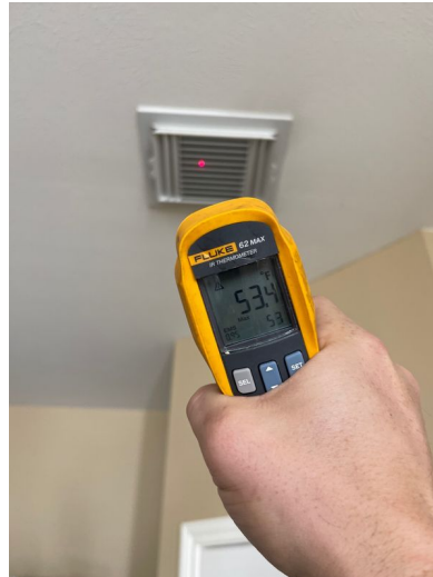
Approximately 53 degree supply air downstairs.
