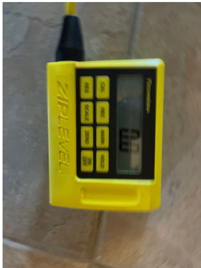
Zero reading taken in middle of foundation.
