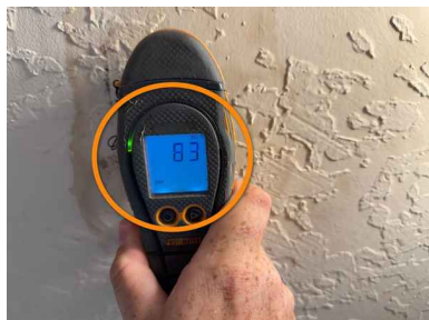
1st Floor Hall confirmed dry
