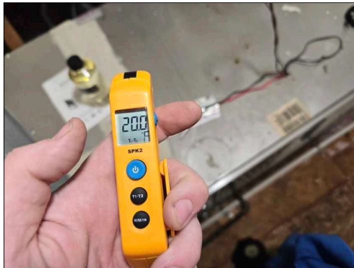
20f delta T across coil is acceptable.
