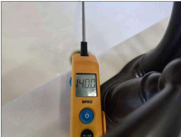
Water heater is set to [140f]. This is high, may scald and be less energy efficient as the normal 120F setting.
